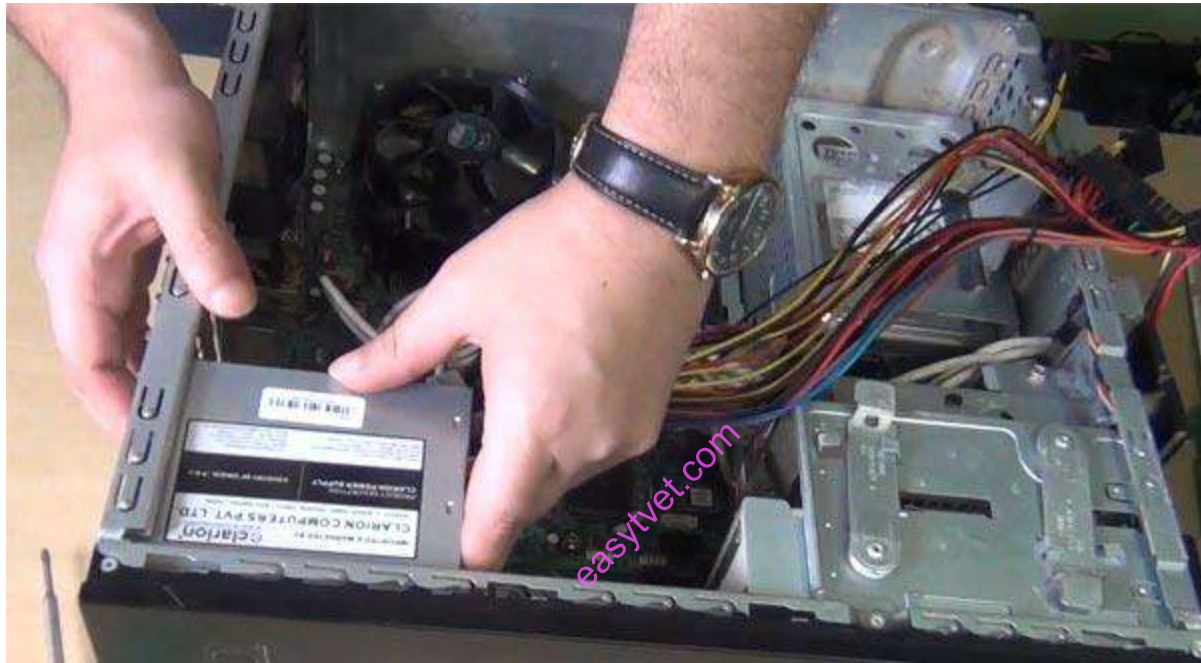
Figure 91 Installing SMPS (Power supply unit)
