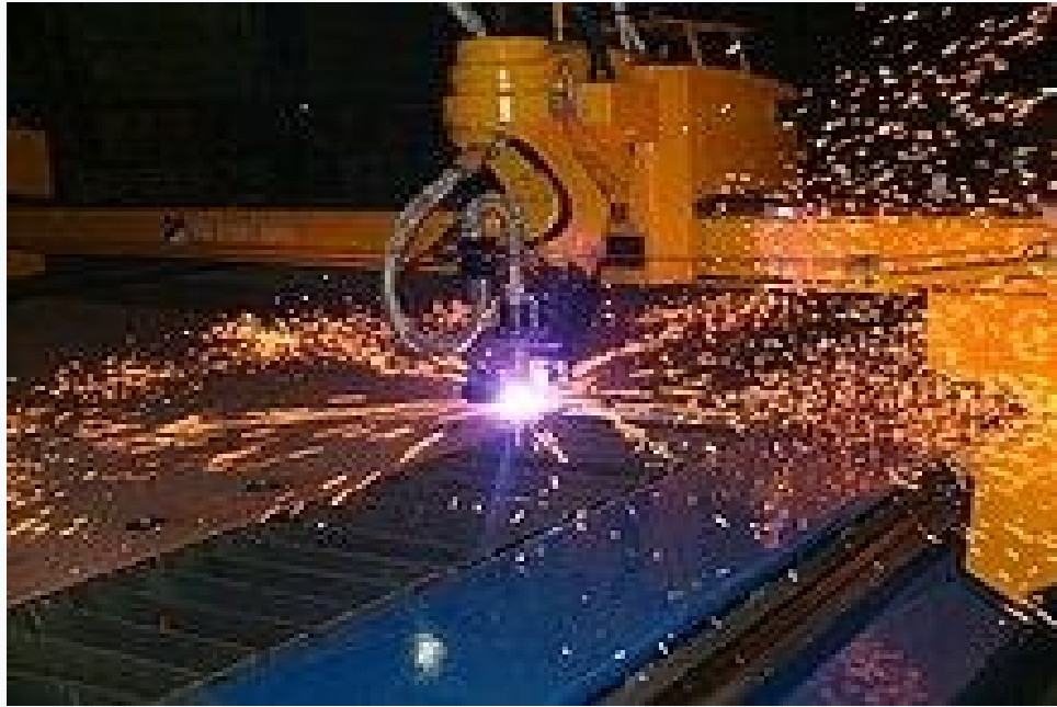
Figure 7: A CNC Plasma Cutting Machine
