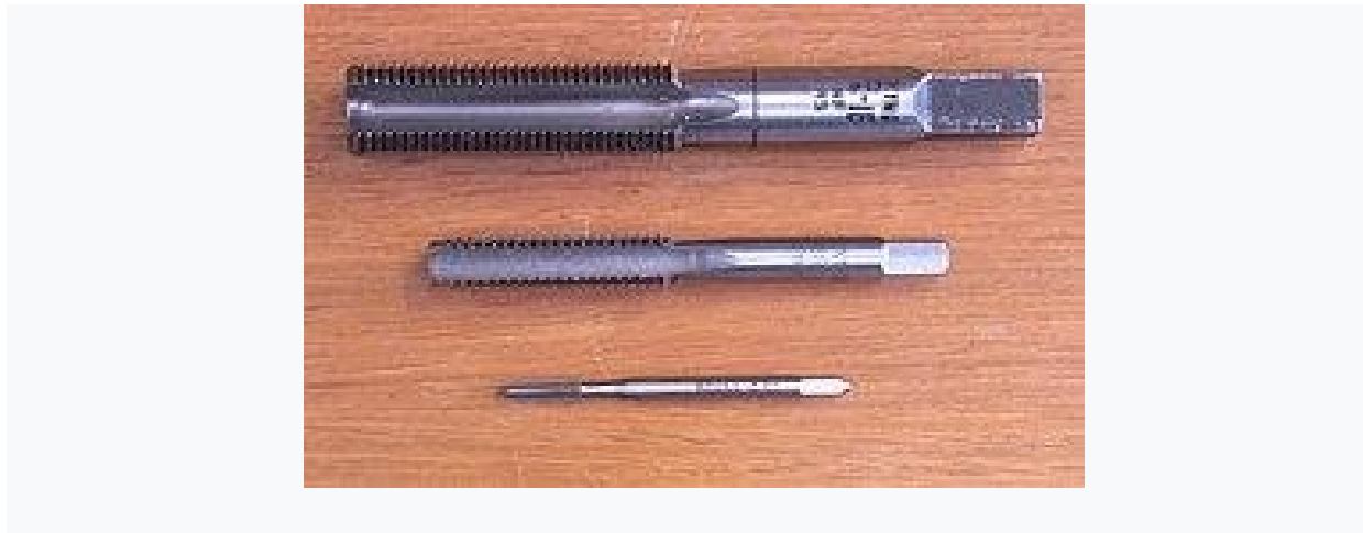
Figure 10: Three Different Types and Sized of Taps
