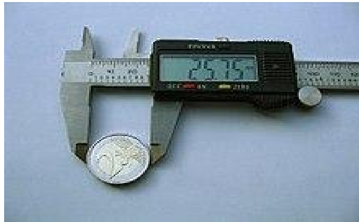
Figure 4: A Caliper for Measuring Length
