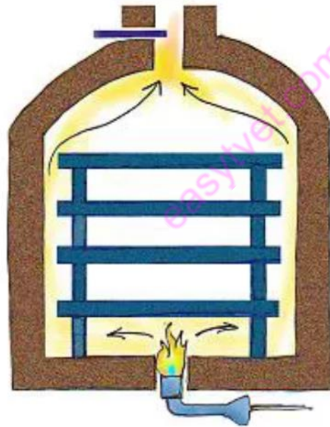
fig. 33. The plan of a typical intermittent up-draught kiln.
