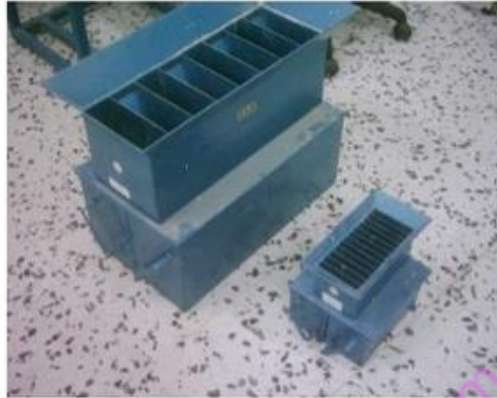
Fig. (1) The sample splitters for fine & coarse aggregates
